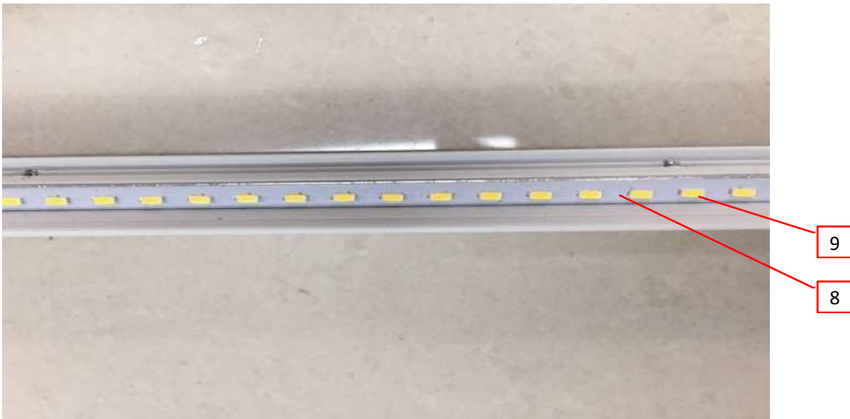
Photo 16 - LED PWB view, LED type 4014, model JS-EP24-60- as representative, only the LED quantity is different with other models
