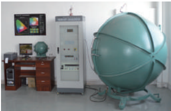
积分球测试 Integrating ball test
